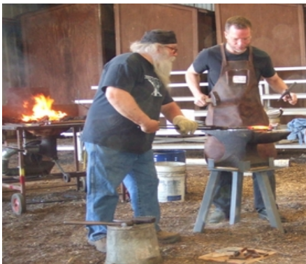
Kim Thomas mentoring punching round pass through holes in round stock
